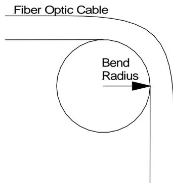
The minimum values for the radius to which cables may be bent can be determined by the following formula:
