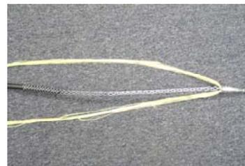
The pulling grip should be sized appropriately for the diameter of the cable. For interlocked and corrugated steel tape cables, the grip also needs to be able to fit the diameter of the outer armored jacket. Kellems pulling grips are recommended. Listed below are sample model numbers for the Kellems pulling grips with and without the swivel eyes and the corresponding cable diameters. Please refer to the Kellems web site for more details.
