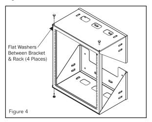
4.6 Be sure to insert flat washers between support brackets and rack frame before tightening thumbscrews.
