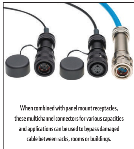
To immediately create a new circuit in a disaster recovery situation, panel mount receptacles with dust caps can be connected to active equipment via standard SC, ST or LC optical fiber interfaces on one end and connected to a deployment reel on the other end.
