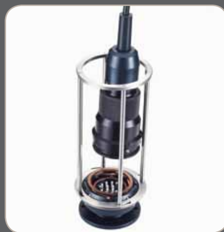
Step 3 The sensing ring (silver color) is pulled in any 360° direction by tethers from within the cabinet. The positive spring pressure ejects the plug within milliseconds.
