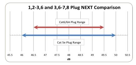
The process has changed slightly during the development of TIA-568-C.2, where the mated performance with limit plugs can be derived mathematically. However, verification of the performance with the high and low limit "plugs" is still required.
