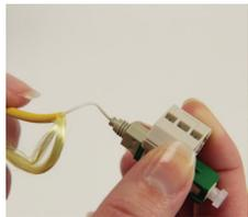
2: Insert fiber into connector making sure the mark is facing up. Create a slight bend to maintain connection.
