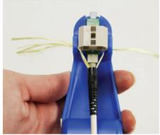
4: Divide the Kevlar® into two portions and place them in the Kevlar® grips. Bring boot forward and screw on halfway.
