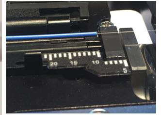
5: Set the fiber on the cleaver at the 10.5 mm cleave length. Cleave the fiber.
