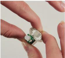
1: Squeeze top and bottom of the wedge to ensure that it is engaged.
