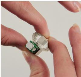
1: Squeeze top and bottom of the wedge to ensure that the wedge is engaged.
