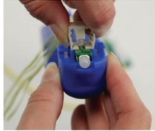
3: Disengage the wedge by squeezing both sides. Remove cable from assembly tool cable grip.
