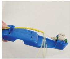
2: Insert the fiber into connector with mark upward until a slight bend is made in the fiber.
