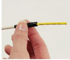
2: Insert the appropriate boot onto the cable.
