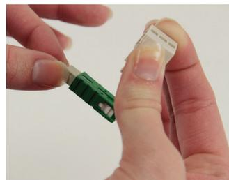
3: Release the wedge clip by squeezing both sides. Remove the wedge clip.
