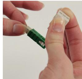
4: Release the wedge clip by squeezing both sides. Remove the wedge clip.
