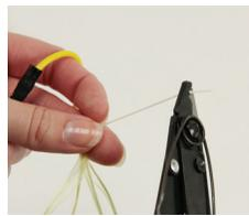
4: Strip off 35 mm of 900 μm and 250 μm coating.
