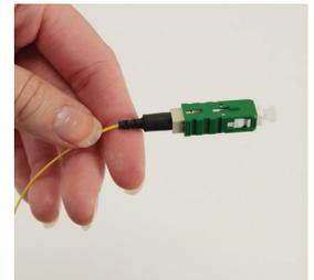
5: Slide the boot onto the connector body. Termination is complete.
