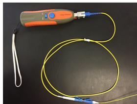
2: Remove the dust cap. Insert the connector into the VFI. Window 1 of the wedge clip will glow red.
