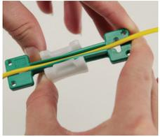
1: Place the cable into the appropriate cable clamp about 10" from the end of the cable.
