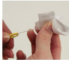
5: Clean the fiber with a lint-free wipe and fiber preparation fluid.
