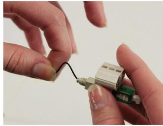
2: Insert fiber into connector. Bring 250 μm protective tubing forward. Create a slight bend in the fiber to maintain connection.
