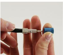
Place the connector into the assembly tool. Squeeze top and bottom of the wedge to ensure that it is engaged. You will not be able to reengage the wedge clip after the housing is applied.
