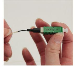
5: Slide the boot onto the connector body. Bring the clear protective tubing over the end of the 250 μm protective tubing. Termination is complete.
