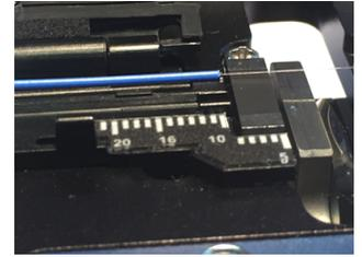
4: Set the fiber on the cleaver at the 10.5 mm cleave length. Cleave the fiber.
