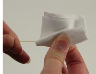
3: Clean the fiber with a lint-free wipe and fiber preparation fluid.
