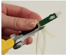
5: Remove from assembly tool. Remove wedge clip completely. Trim excess Kevlar® using the Kevlar® scissors.
