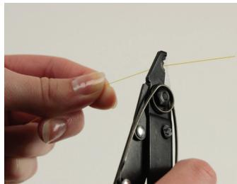
2: Strip 35 mm of 250 µm coating from the fiber.
