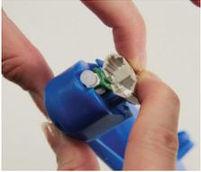
1: Place the connector into the assembly tool. Squeeze top and bottom of the wedge to ensure that it is engaged.
