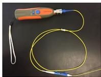
3: Insert the fiber into the connector with the mark facing up. The light will dim when a connection is made.
