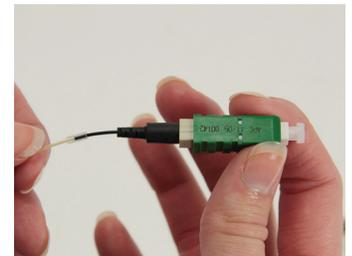
4: Slide the boot onto the connector body. Bring the clear protective tubing over the end of the 250 μm protective tubing. Termination is complete.
