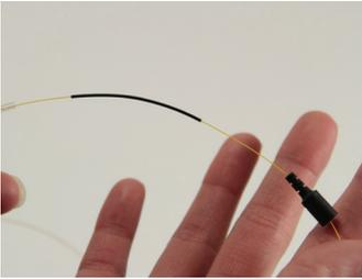
1: Insert the clear protective tubing, 250 μm protective tubing and 900 μm boot onto the fiber.
