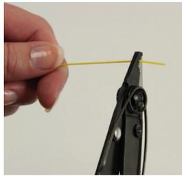
3: Strip 35 mm of 900  $\mu\text{m}$  and 250  $\mu\text{m}$  coating off.
