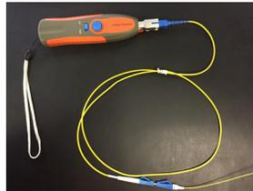
3: Insert the fiber into the connector. Bring 250 μm protective tubing forward. The light will dim when a connection is made.
