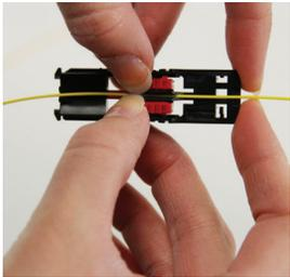
1: If you are using a 900  $\mu\text{m}$  fanout/breakout kit, place into 900  $\mu\text{m}$  cable clamp about 10" from the end of the cable.
