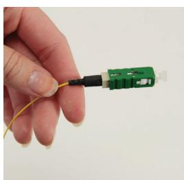
5: Slide the boot onto the connector body. Termination is complete.
