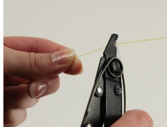
2: Strip 35 mm of 250 μm coating from the fiber.
