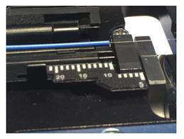
6: Set the fiber on the cleaver at the 10.5 mm cleave length. Cleave the fiber.
