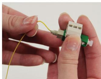
2: Insert the fiber into the connector with mark facing up. Create a slight bend in the connector to maintain connection.
