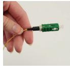
**5**: Slide the boot onto the connector body. Termination is complete.
