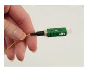
**4:** Slide the boot onto the connector body. Termination is complete.
