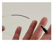
1: Insert the clear protective tubing, 250 µm protective tubing and 900 µm boot onto the fiber.
