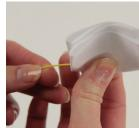
**4:** Clean the fiber with a lint-free wipe and fiber preparation fluid.
