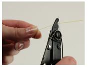
2: Strip 35 mm of 250  $\mu$ m coating from the fiber.
