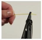
3: Strip 35 mm of 900  $\mu$ m and 250  $\mu$ m coating off.
