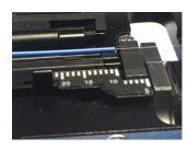
**4:** Set the fiber on the cleaver at the 10.5 mm cleave length. Cleave the fiber.
