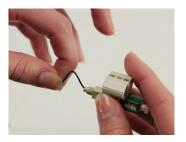
2: Insert fiber into connector. Bring 250 µm protective tubing forward. Create a slight bend in the fiber to maintain connection.
