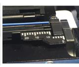
**5:** Set the fiber on the cleaver at the 10.5 mm cleave length. Cleave the fiber.
