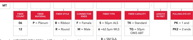
Example: MT12RBM5TK-03PK = MT riser cable assembly,
