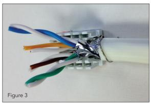
4.4 Insert conductors into slots and trim excess wires using diagonal cutters with flush cutting edge. See Figure 4.
