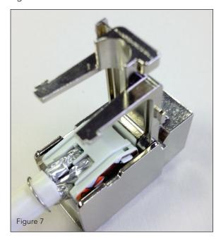
4.8 Ensure drain wire is inserted through slot in connector body and is making contact with the cable strain relief on hinged cover. Insert cable tie through slot and tighten around drain wire and cable. See Figure 8.
