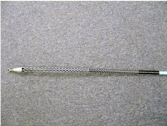
Figure 4: Pulling Grip Installed on Cable
