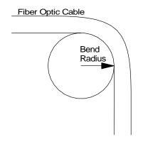
The minimum values for the radius to which cables may be bent can be determined by the following formula:
