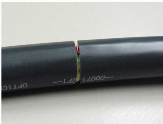
Figure 1: Ring Cut in Cable at Marked Distance
