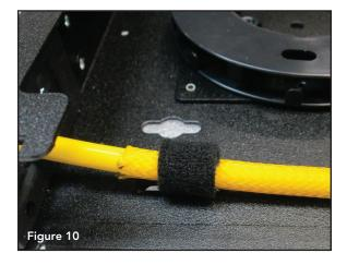
7.11 Secure the cable with tie wraps or velcro to the Strain Relief Bracket (if used). See Figure 11.
