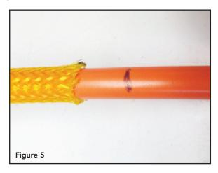
Strip outer jacket back to the mark on the cable exposing the 900 micron buffer fiber. Slide the nylon protective sock up over the 900 micron fibers until it is covering only the last inch of the jacketed cable.
