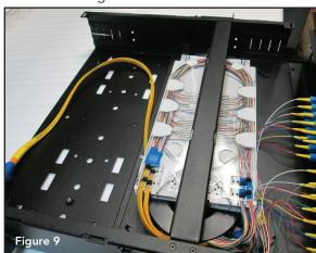
7.10 Route cable through the cable entry port until the mark on the cable is even with the velcro/cable tie mount. Secure the nylon protective sock on the cable and secure the cable with velcro tie wraps to velcro/cable tie mount. See Figure 10.
