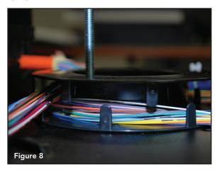
Taking care not to pinch or overbend the fibers, slide the tray back into the enclosure until it locks into forward position making sure there is enough slack cable to fully extend the tray forward. See Figure 9.
