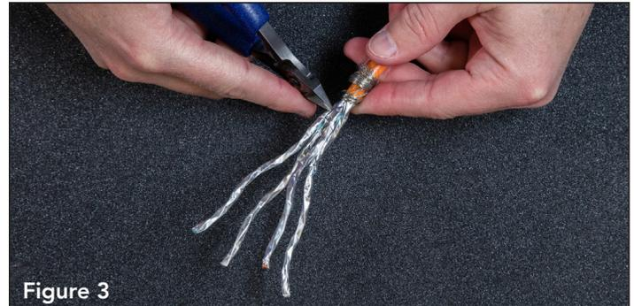
4.4 Sort pairs as shown for T568B wiring. Untwist and smooth conductors to prepare for insertion into wire manager. Do not disturb the pair twist within the cable jacket. See Figure 4.
