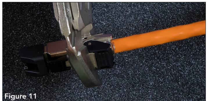
4.11 Fully depress black strain relief until it is firmly against cable jacket.
