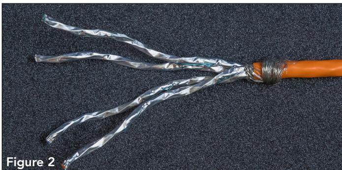
4.3 Score and remove foil screen from each pair. If using an Sc/FTP cable, score and remove overall foil from pairs. See Figure 3.
