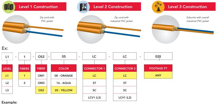
L1-1-OS2-05-LC-LC-025 = Level 1, 1 Fiber, Single Mode, Yellow, LC, LC, 25 Feet L1-2-OS2-05-LC-LC-025 = Level 1, 2 Fiber, Single Mode, Yellow, LC, LC, 25 Feet
