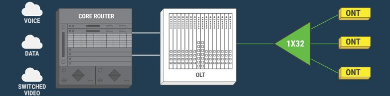
The OCC POL Solution ensures network traffic is transported between these devices over a passive optical fiber infrastructure that generally consists of the following components:
