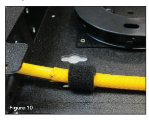
7.11 Secure the cable with tie wraps or velcro to the Strain Relief Bracket (if used). See Figure 11.
