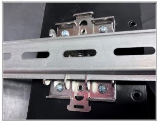
3. Once the clip is securely mounted, the panel can slide along the DIN rail and positioned as required.
